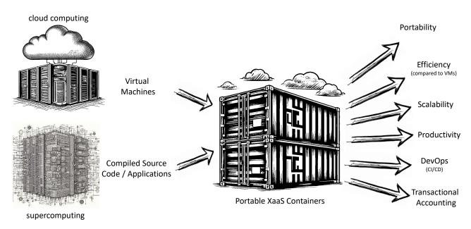
Figure 1: Both Cloud and HPC converge to containers as an application and service deployment model. Containers bind all dependencies and system aspects (users, rights, etc.) into a single portable unit that can be flexibly deployed. XaaS enables HPC features for such containers.
