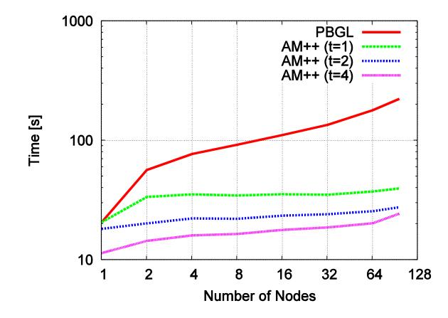
Single-data-rate InfiniBand, dual-socket dual-core, 2<sup>24</sup> vertices/node, degree 4
